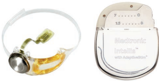
Figure 6.2 Two examples of medical implants that use enclosures. (Left) Argus II Retinal Implant (external system not shown). Feedthroughs for the Argus II are on the other side of the silver case and are not visible in this picture. (Right) Medtronic Intellis — smallest fully-implantable spinal cord neurostimulator.
